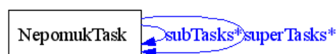
Figure 6.9: The Task Schema allows for references to Super-tasks and Sub-tasks. On the instance level, a task hierarchy looks like in Figure 6.10.
